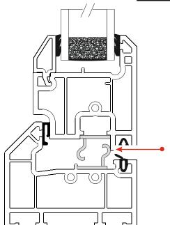
STAY GUARD ELITE SG037 on outer frame and sash for all types of stays to include Egress/Easy Clean
